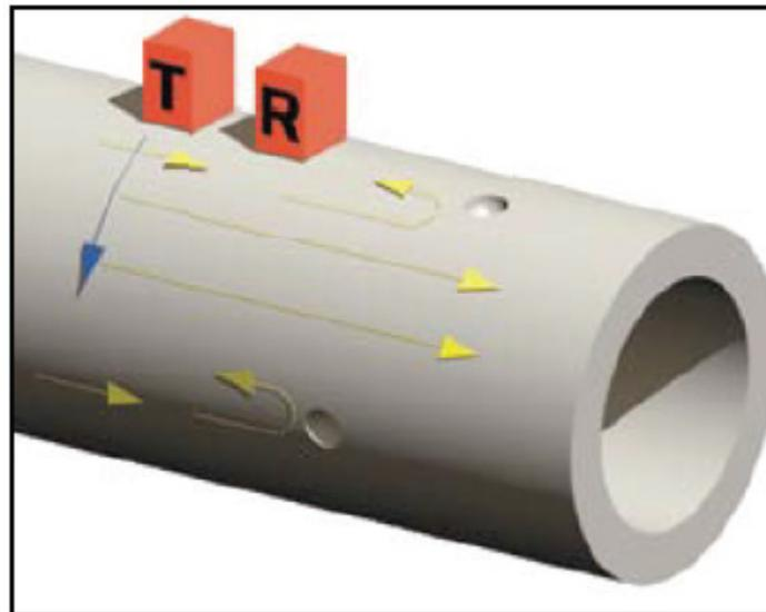
**Figure 3** Ultrasonic EMAT method for circumferential scan of pipe.
