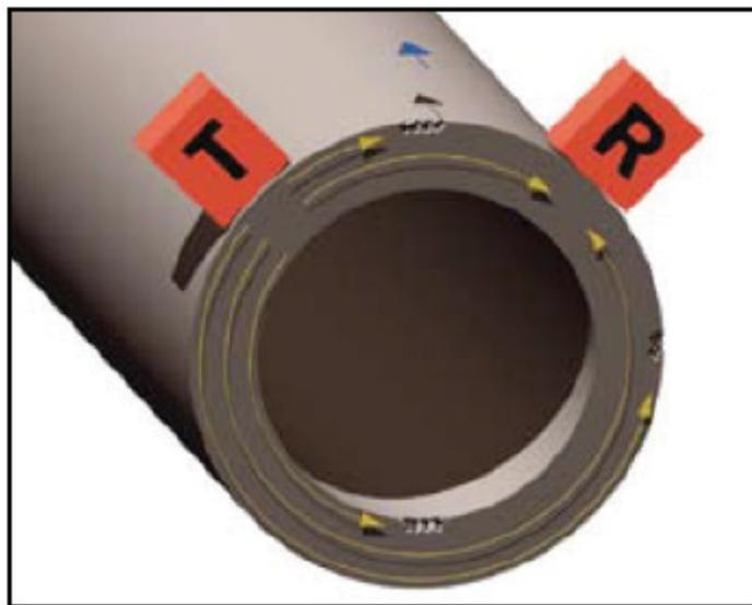
**Figure 2** Ultrasonic EMAT method for axial scan of pipe.
