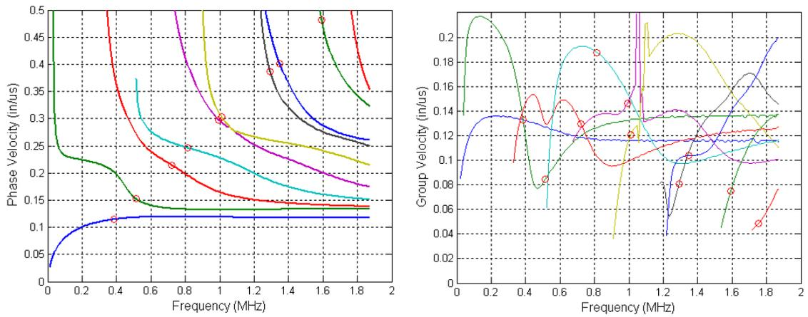
Figure 11: Phase and Group Velocity Curves used to determine frequency and wave mode for a particular tube diameter and wall thickness
