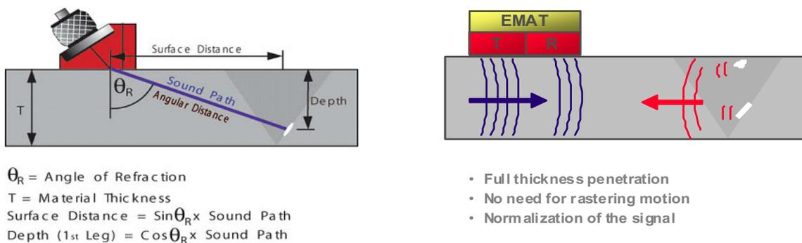
Figure 6: Comparison of angled beam and volumetric guided wave methods for Weld inspection
