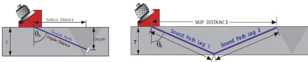
Figure 4: ID/OD weld defect detection using "half skip/Full skip" method
