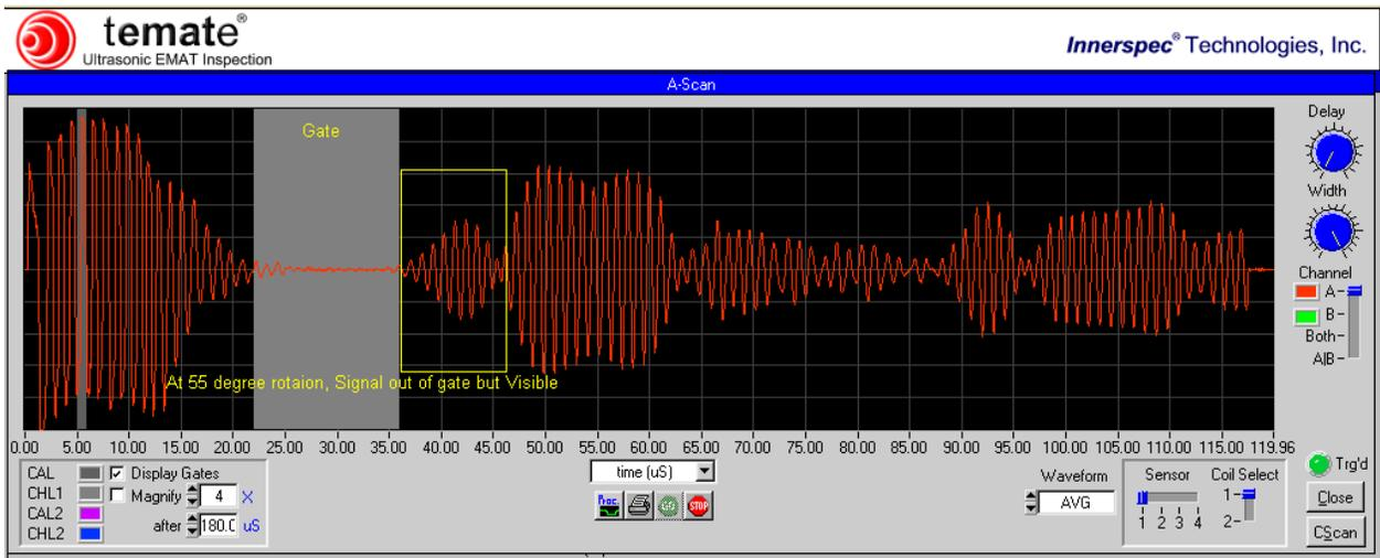
Figure 8: Defect is Easily Detected +/- 22.5° from the Normal
