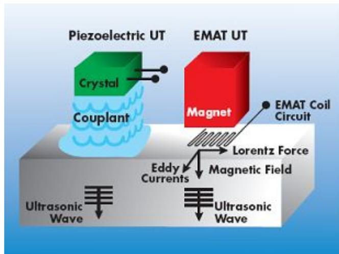
Figure 5: Comparison of piezoelectric and EMAT sound generation
