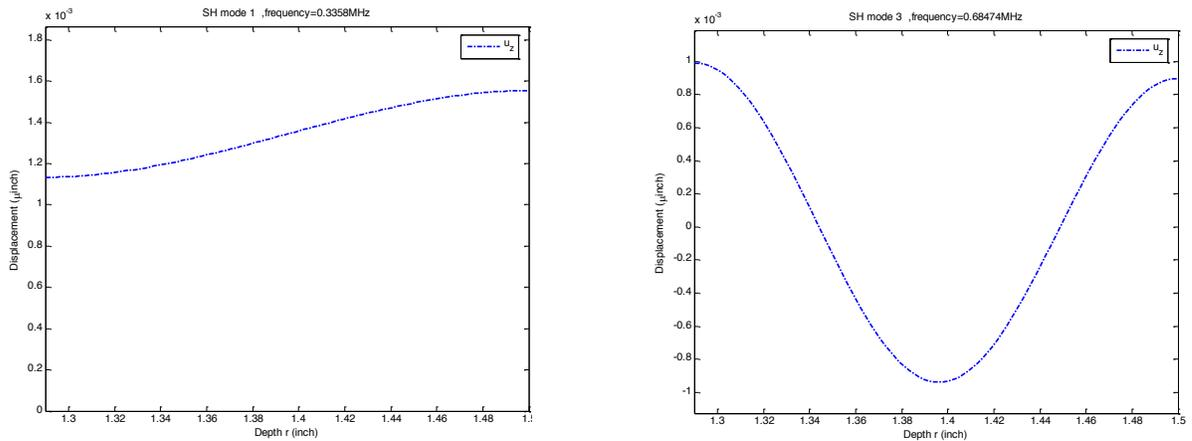
Figure 12: Wave displacement curves. Left Curve shows good amplitude of particle motion from ID to OD surface. Right Curve shows good ID and OD amplitude but poor Mid-wall sensitivity (A flat line represents equal sensitivity across the weld)
