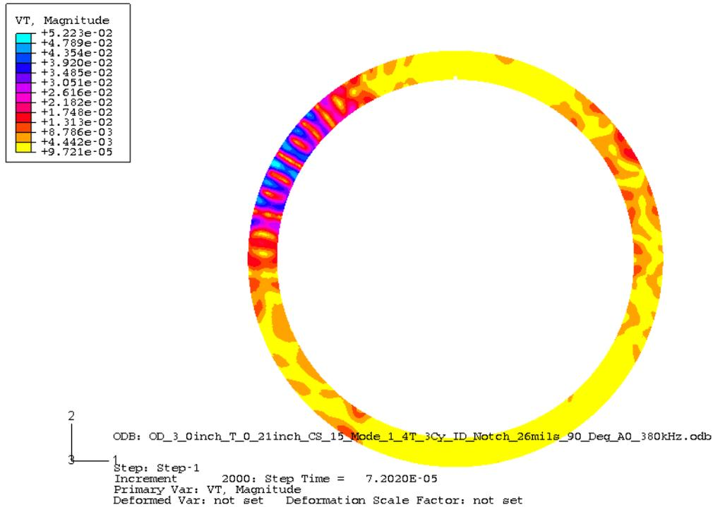
Figure 13: FEMM Modeling of Wave Mode Reacting to ID, OD and Mid-Wall Defects to Verify Sensitivity
