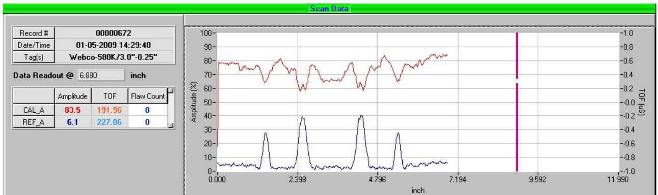
Figure 14: Tube with ID/OD Notches Verifies Modeling
